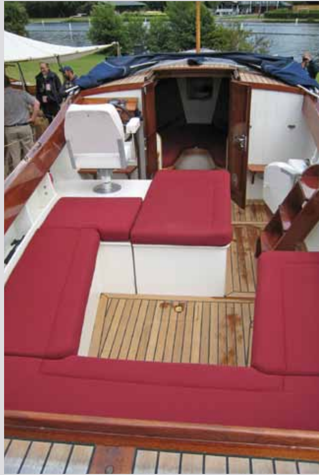
In the cockpit and down below on Morgana. She was built using modern wooden boat construction methods – epoxy glued western red cedar strip planking over CNC-cut moulds and glassed inside and out – by Win Cnoops at Star Yachts, Bristol. She's a Bristol 22, designed by Andrew N Wolstenholme who also took these pictures at the Thames Traditional Boat Rally in 2011.
