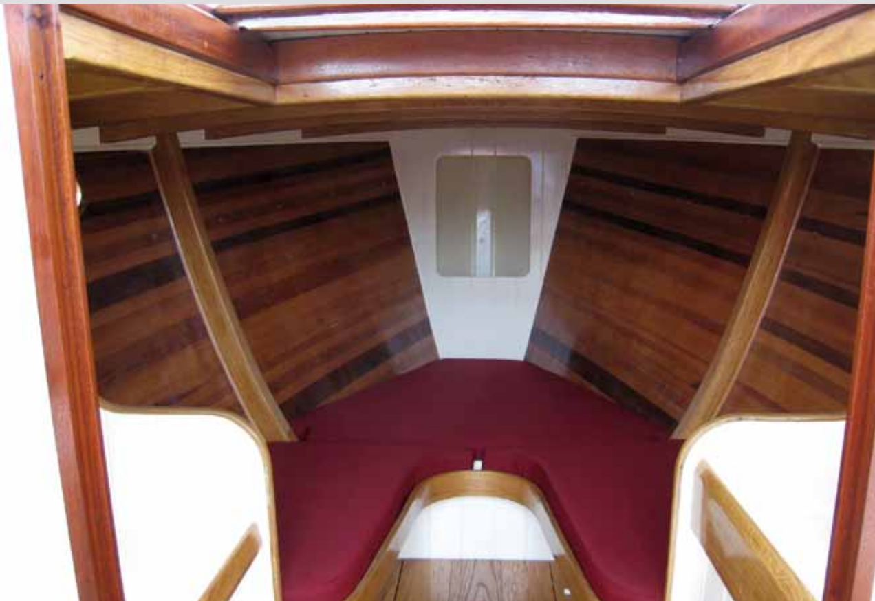
In the cockpit and down below on Morgana. She was built using modern wooden boat construction methods – epoxy glued western red cedar strip planking over CNC-cut moulds and glassed inside and out – by Win Cnoops at Star Yachts, Bristol. She's a Bristol 22, designed by Andrew N Wolstenholme who also took these pictures at the Thames Traditional Boat Rally in 2011.
